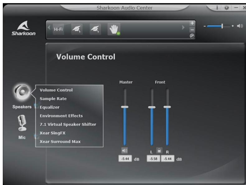
Through the Sharkoon Audio Center, control the volume of the RUSH ER40 speakers, make changes to the sound via the equalizer, access a variety of pre-installed effects, and configure the simulated position of the 7.1 surround sound. To access the individual menu items, right-click on the speaker symbol on the left side of the software.
